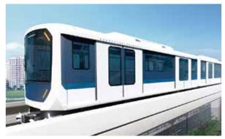
The 8 car AGT train of type A, which has the same width as the subway shown on the left, has almost the same passenger capacity as the 6 car subway train.
